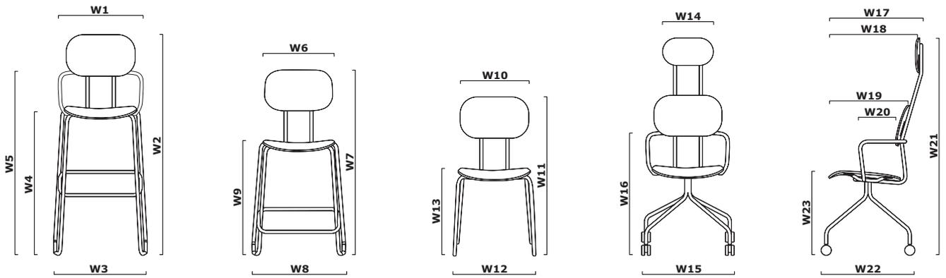
W1 - 535 | W2 - 1175 | W3 - 517 | W4 - 820 | W5 - 1025 | W6 - 420 | W7 - 995 | W8 - 517 | W9 - 640 | W10 - 390 | W11 - 817 | W12 - 458 | W13 - 462 |
