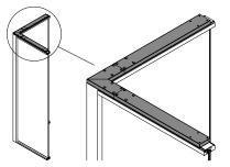
If required, it is possible to order self-supporting walls - independent from a ceiling - in the desired height by fixing on the top of the head tracks a 100×30mm tubular metal profile - prices available in the Accessories section. Self-supporting walls are stable and safe if all junctions are achieved using aluminium tracks whilst avoiding glazed junctions made with polycarbonate dry joints
